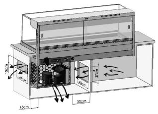
Do not install hot equipment inside the condensing unit space. Leave the back of the cabinet open if possible.
